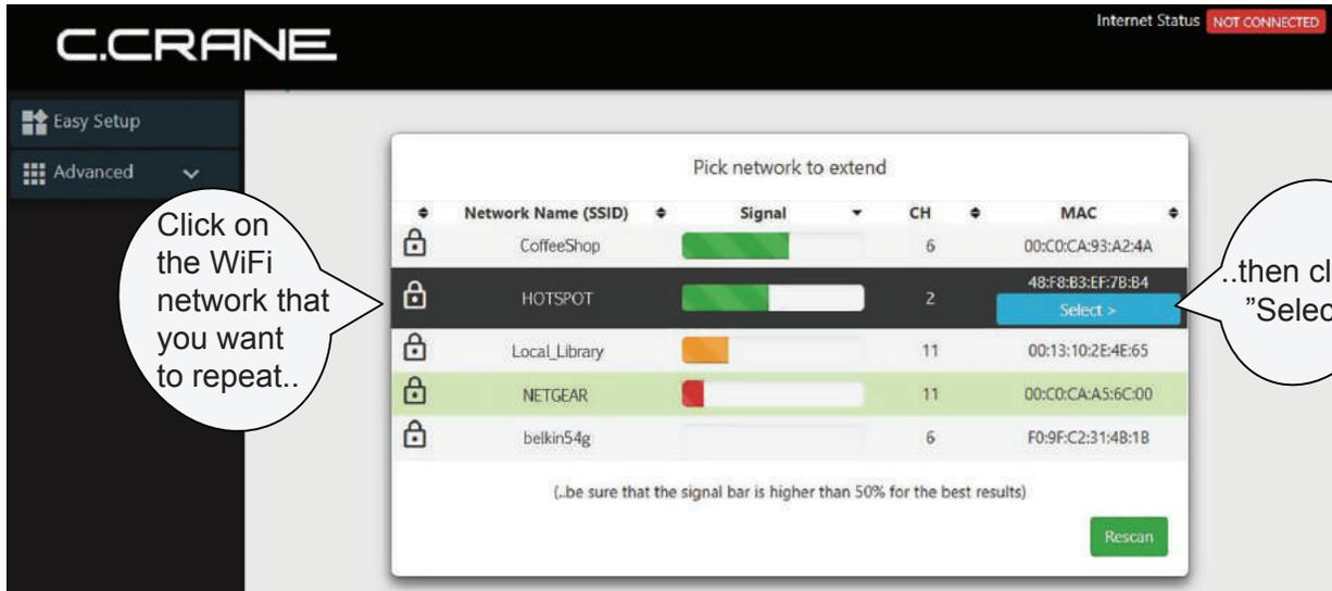
**NOTE:** For best performance, your signal should be higher than 50%. For a better signal, try adjusting the orientation and placement of the USB antenna - then click “Rescan” to see if the signal is higher.
