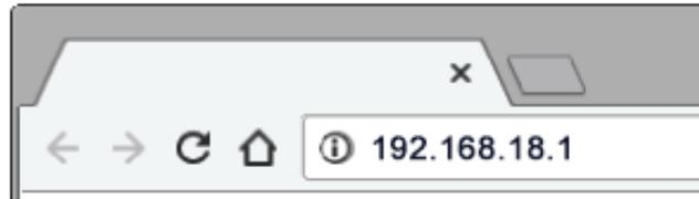
**NOTE:** At this point you are connected to the CC Vector but your browser will likely tell you that you are not connected to the internet. This is normal because the CC Vector is not yet setup. Continue with the setup.
