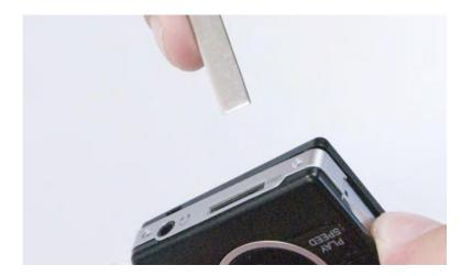
4. Slide the tool around to the bottom of the unit while keeping the tool 1/16 inch into the separation. Continue this same technique while rounding all the edges of the case.
