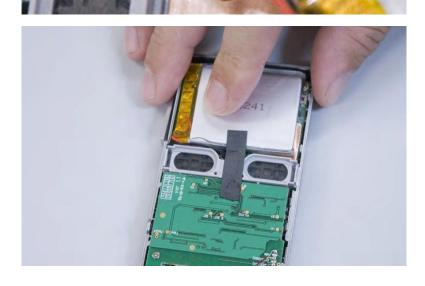
11. Using both hands, gently apply pressure to the back cover until the case is fully clipped together.
