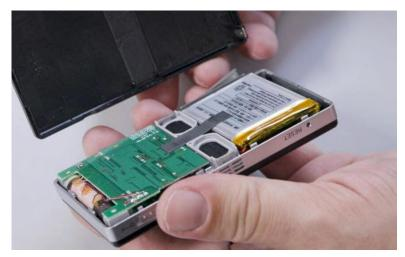
7. Remove the old battery, along with the tape.
