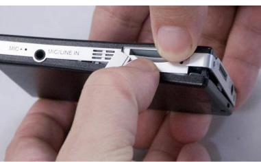
Insert a flat metal tool with smooth edges (like a butter knlfe) 1/16 inch into the separation.
