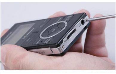
2. Open the cover to the SD Card slot and, using both thumbs, separate the case by 1/8 inch.
